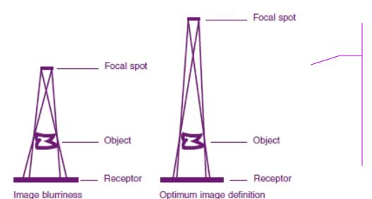
Contrary to appearances, the compact tube implements extensive internal collimation of the X-ray beam, giving a minimum source-skin distance of 30 cm. This gives sharper images and improved detail with respect to traditional X-ray units.
